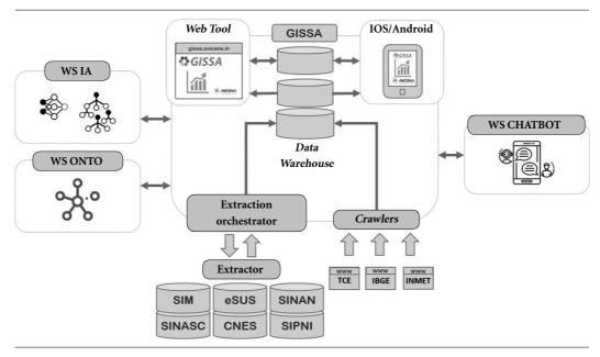
Figure 1. Components of the current system architecture.
