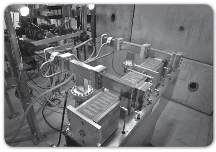
This is one of the first modules of a compact linear accelerator, used for hadron therapy
